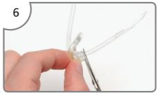
Cut the tapered end as close to the ear mould as possible. Make sure this is smooth as it is the part that goes in your ear
