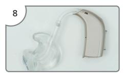
Make sure the mould bends in the right direction as shown
