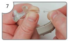
Push the end of the new tubing onto the elbow of the hearing aid
