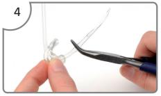
Pull tapered end through until the bend reaches the earmould and the tubing is pointing 90° towards the top of the mould
